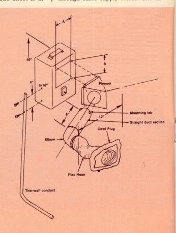
sign may be adapted to any small heater of this type. With a small heater such as this it is important to put all of its output in and around the engine. Remember to keep a close fit of warm air ducts to the cowl openings and short duct runs.
